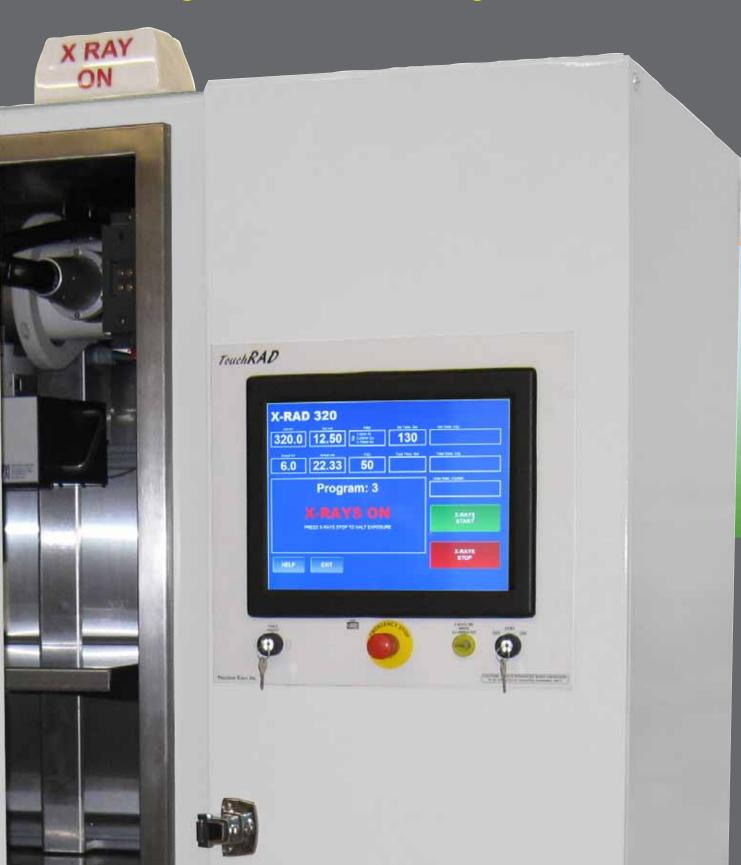
The X-RAD 320ix is a self-contained X-ray system for delivering a precise radiation dosage to specimens in a biological or small animal research laboratory.
